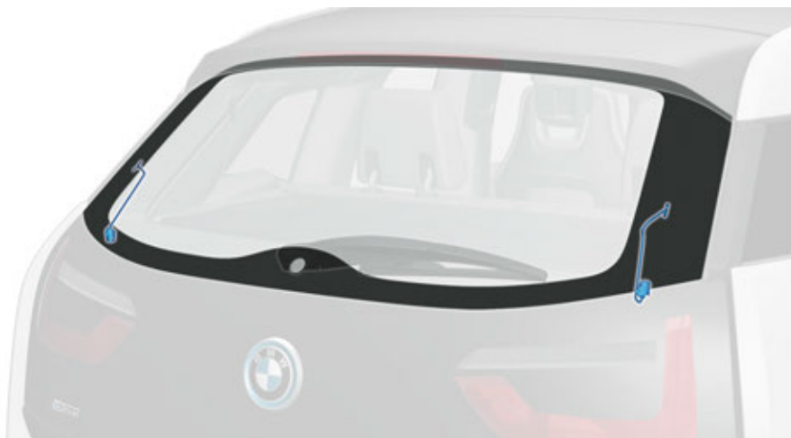
Rear window with electrical plug connections
